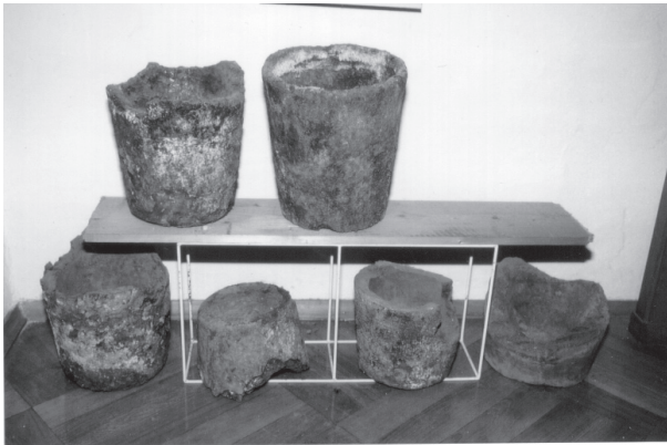
Figure 6: Original crucibles from the brass foundry in Rodewisch-Niederauerbach (found after 1950 during road construction work). Display in the Göltzsch Museum, Rodewisch, Saxony. (Photo by the author.)
