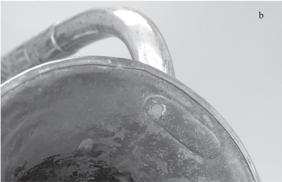
Figures 14a–b: Rodenbostel slide trumpet, (a) with two holes in the garland (see arrows) and (b) the patch covering them on the inside of the bell (NMM 13505).
