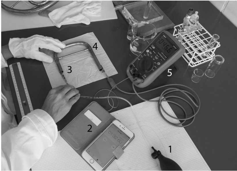
Figure 3: Experimental arrangement for the in-situ measurements of corrosion potential. 1: hand pump; 2: chronometer to record values at precise times; 3: PVC tube in which the sensor and a reference electrode were mounted; 4: tuning slide used as a working electrode; 5: voltmeter to measure potential values.
