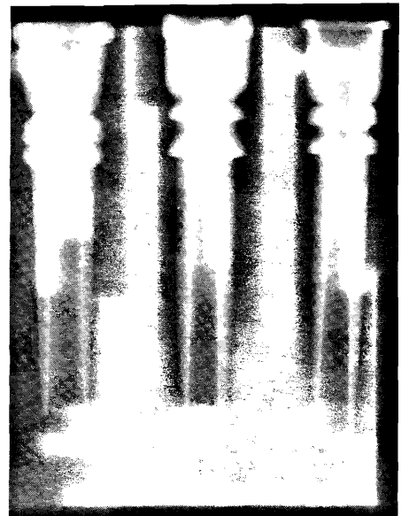
Figure 5. X-ray of three mouthpieces. From left: one of Swiss design, and two by the author. For purposes of scale in the photograph, the center mouthpiece is 11.8 cm long, and has a 4.0 mm bore.
